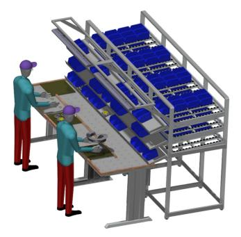
Structured material flow via a FIFO gravity flow rack in an I-shaped production line, in which up to two workers can assemble power packs in a one piece flow system.
