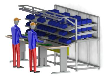
The FIFO gravity flow rack is filled from behind by the warehouse staff. The inclined base of the shelves means the parts fall into the material containers to the assembly workers on the production line, where they are fitted according to the "first in, first out" principle.
